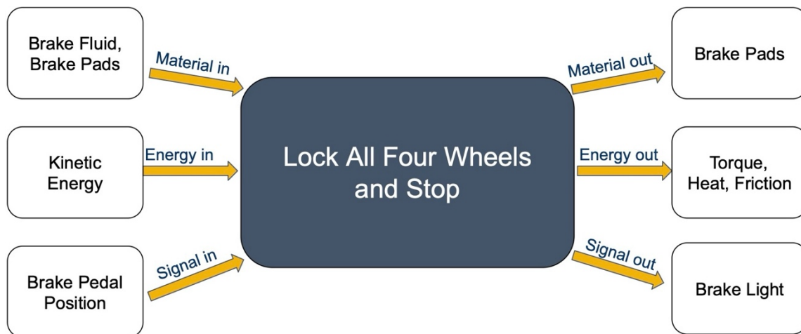
Figure 10: Black Box Model of Brake System
