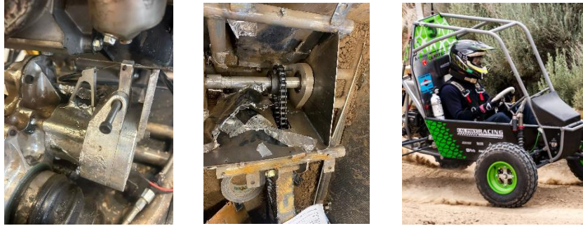
Figure 3: 4WD System and Front Gear Box from previous NAU teams and Cal Poly Racing
